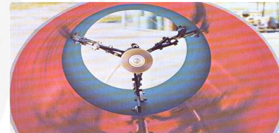
•Orbiter: coating equipment inside pipe
